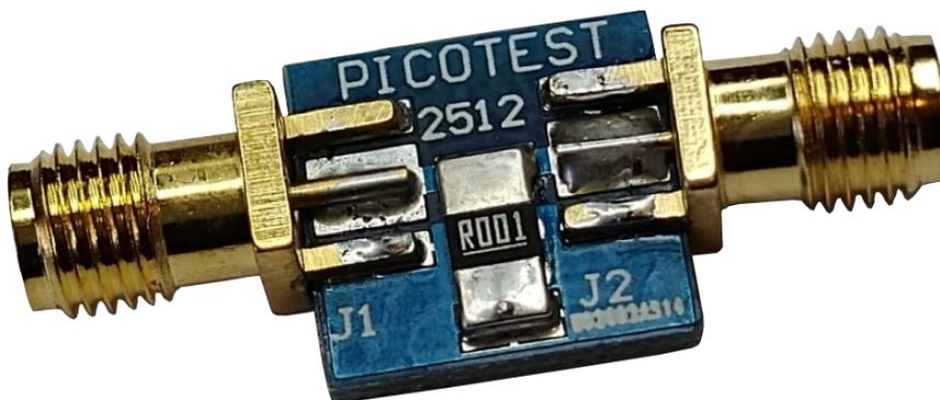
**Figure 10: Measured 1mΩ resistance mounted on one of the Picotest DTBK01 test boards.**
